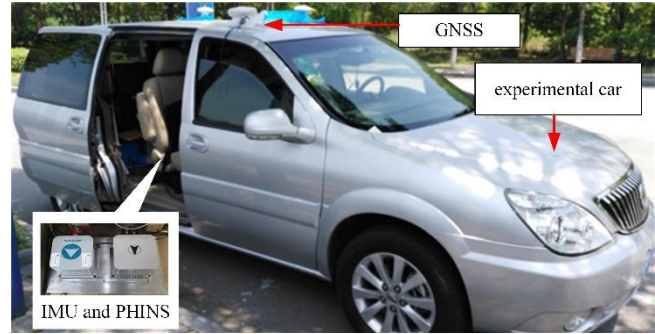
Fig. 14 A schematic of the experimental car The trajectory of the car is shown in Fig.15.
